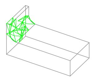
What: Calculate the distortion and stretch of the elements, listing the elements below selected threshold values.
