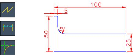
Why: The dimensions of this part and the meshing parameters used later will result in distorted elements. What: Extrude 50mm and name the part.
